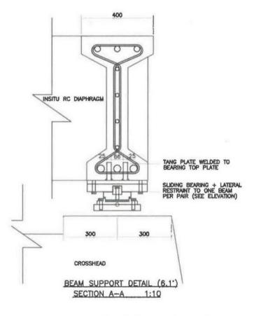
Figure 3 Cross-section of rail support beam at bearing location (guided bearing shown).
