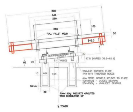
Figure 13 Option for dealing with misalignment if keeping inclined bearings – use of extended bearing top plate (with possible bolt into site-drilled hole in beam soffit plate)
