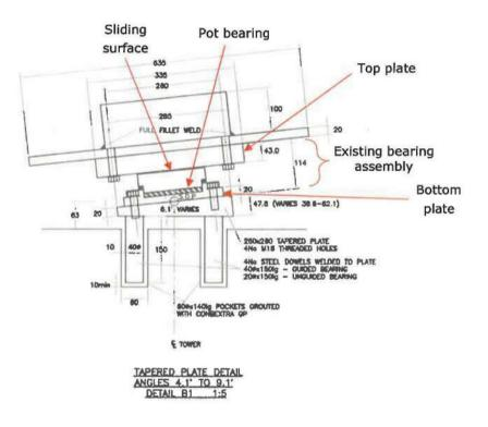
Figure 1 Current bearing detail at piers with tapered plates (tapered plates used at 62 No. locations)
