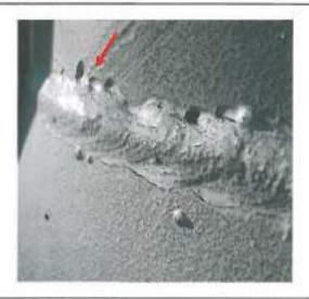
Photographic record showing Undercut on Left hand side (9 o'clock position) on tower 11.
