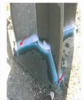
Photographic record of Base Plate and Anchor Bolts on Tower 1. Indications found on both Stiffener Webs facing down-hill.
