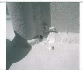
Photographic Record showing Porosity on Stiffening Web facing up-hill (12 o'clock) on Tower
