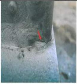
Photographic record showing 7mm Indication on right hand side Stiffener facing down-hill on Tower 2 indicated by red arrow.
