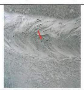
Photographic record showing Porosity in "Cone to Tower" weld at 6 o'clock (downhill) on Tower 2.
