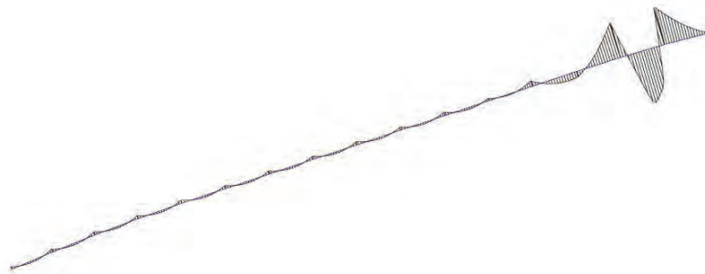
Figure 5-3 Typical line beam bending moment for a typical live load plus superimposed dead load case
