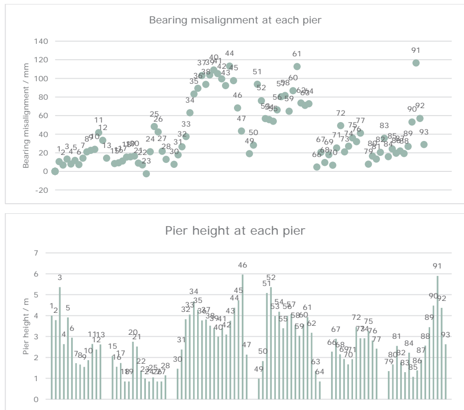
Figure 6-4 Longitudinal displacement of bearings along viaduct length at a reference temperature of 0°C and pier heights for comparison.
