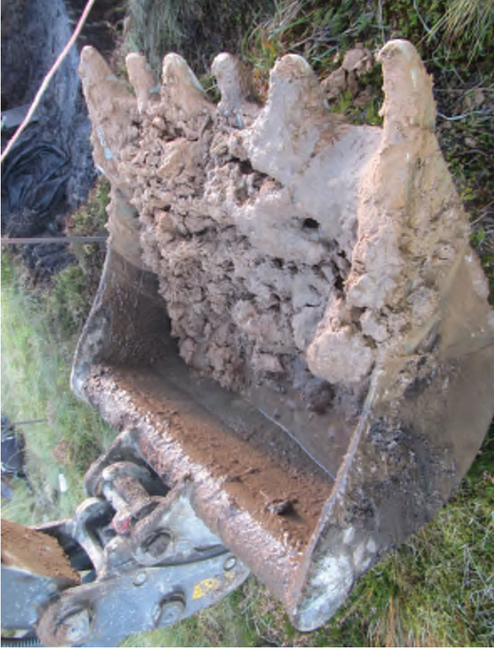
1.95-2.2m Yellow brown slightly clayey silty SAND with occasional lenses of firm sandy silt up to 5cm in thickness. Assessed as loose. (Alluvium)
