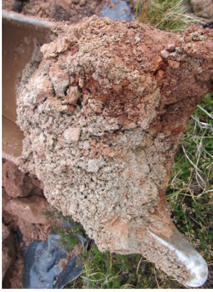
0.0-1.65m Light grey and orange/red brown gravelly SAND with trace silt and occasional cobbles and boulders. Assessed as medium dense. Gravel, cobbles and boulders are sub-angular to rounded of granite lithology occasionally decomposed to residual soil. (Glacial Deposits).
