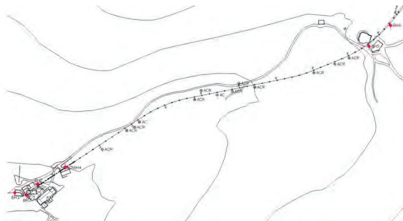
Figure 2-2 1998-99 Ground investigation borehole location plan.
