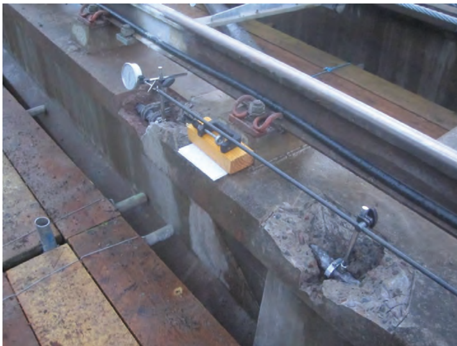
Figure 2 Type 2: General setup for reinforcement deformation tests
