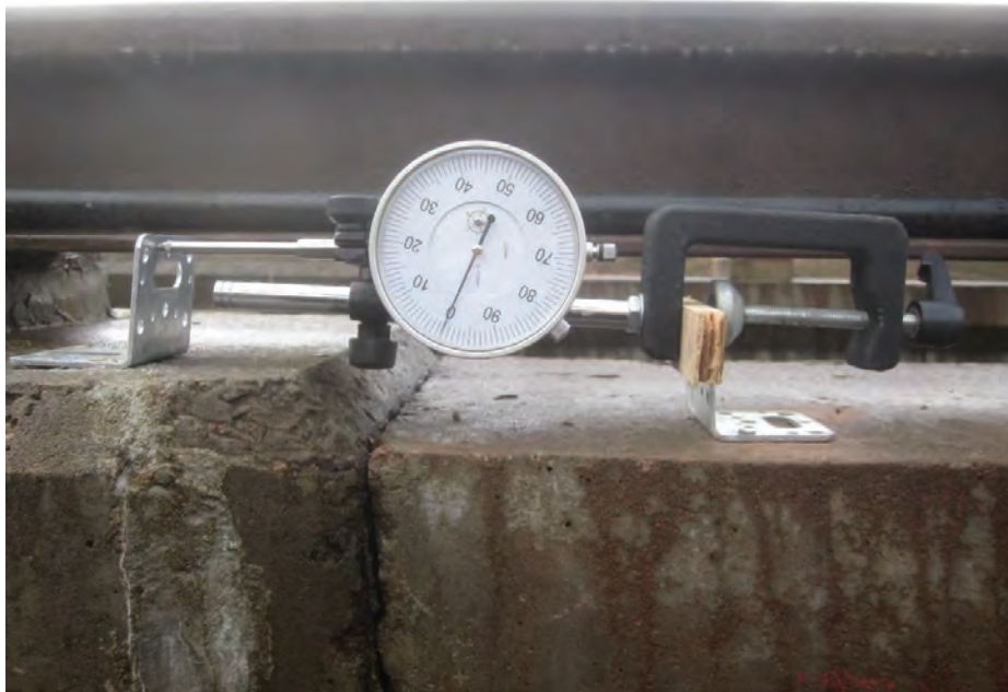
Figure 1 Type 1: General setup for crack width measurement tests
