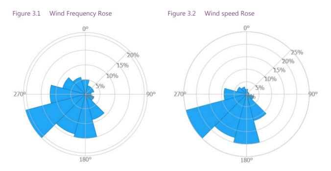
As is common for UK wind turbines, the prevailing wind direction in South-West.
