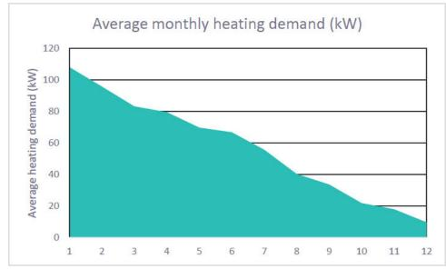
This data suggests that a boiler sized at about the same rating as the existing boiler in the day lodge (120 kW) would be adequate to meet the total heating needs of both the Day Lodge and the Base Station buildings. This includes the current heating requirements met by electrical heating.
